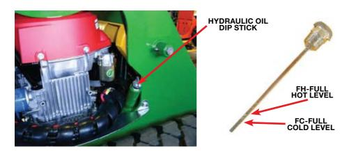
Inspect all hydraulic hoses, tubes, fittings, valves and rams for leaks and damage. Tighten loose fittings and replace damaged components.
