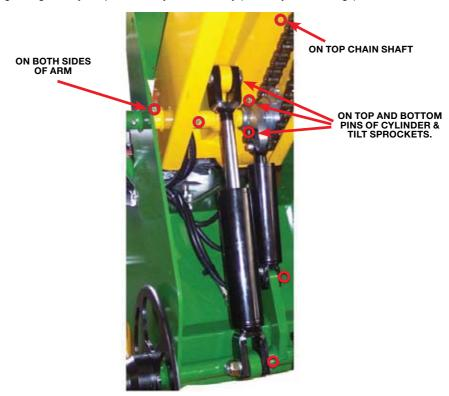
Ogrease Nipples Regreasing during the day of operation may be necessary (See Daily Checks).
