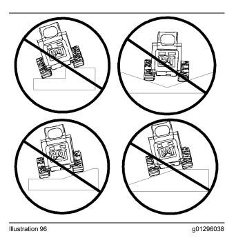
NOTICE Avoid operating this machine on transitions. Operating this machine on transitions may cause the tracks to derail.
