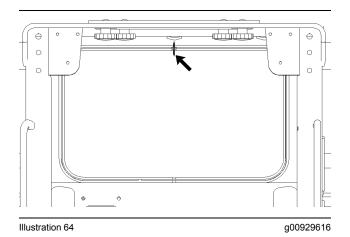
The opening in the rear of the machine serves as an alternate exit. The window (if equipped) will need to be removed in order to use the alternate exit.
